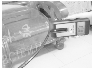
figure 1: Correct method of placing Model 1000 on glass.
